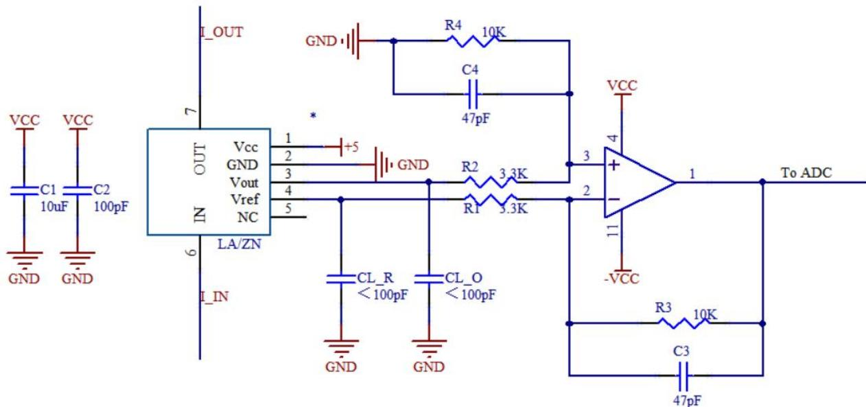
Typical application circuits for STB-LA current sensor. The magnification can be estimated as  $M = R4 / R2$  with the condition of  $R1 = R2$ , and  $R3 = R4$ . The magnification in the circuit above is around 3. The capacitive load of  $V_{out}$  and  $V_{ref}$  should not exceed 100pF to avoid oscillations.
